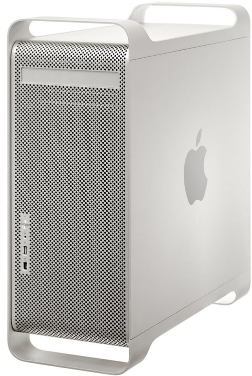
The Apple Power Mac G5 which, in 2004, came as standard with 256 MB of RAM and a 80 GB hard disk drive.
