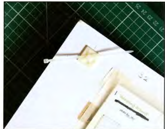
Rear fixing – shows the cleats and zip ties
