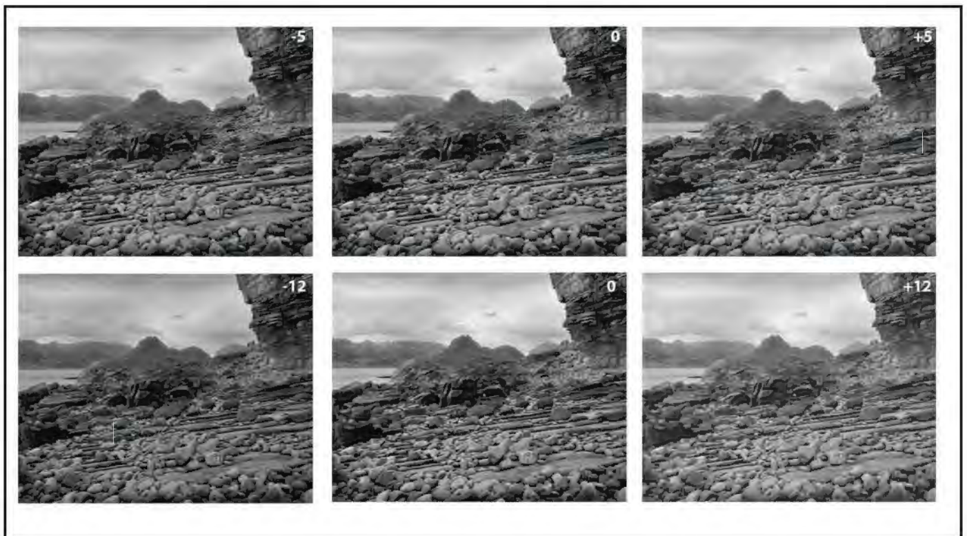
Figure 5: The test print adjusted to display the levels of error found during testing, ±5 in the top row, ±12 in the bottom row
