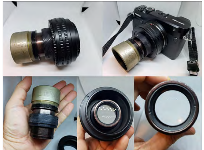
The custom modified 70mm projection lens and Fujifilm G-mount adaptor used for the image below
