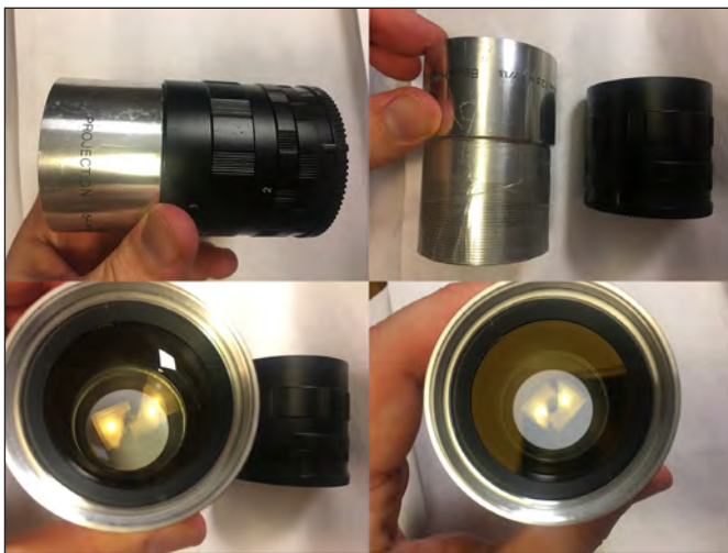
The custom modified Kinostar 80mm projection lens and Sony E-mount adaptor used for the image above
