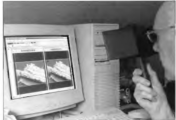
ScreenScope viewer for side-by-side view of larger prints or screen images. With the computer program 3D Viewer ( www.stereoaid.com.au ) it is possible to zoom into selected regions of the image, still retaining the 3D effect.
